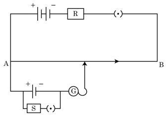
Keeping other things unchanged (a) X increases the value of resistance R, (b) Y decrease the value of resistance S in the set up. How will these changes affect the position of null point in each case and why?
